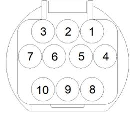
NOTE: Looking from rear of connector on vehicle side.
